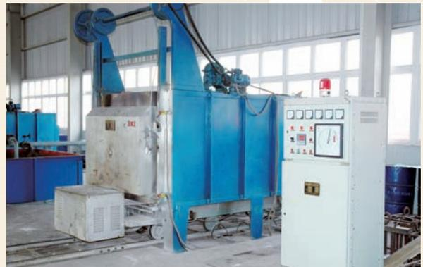
RJ2-75-6台车式电阻炉
