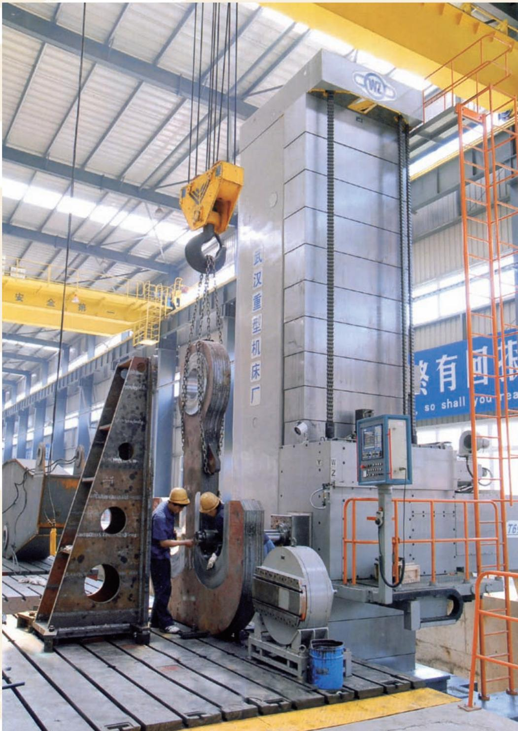
大型数控落地铣镗床 Large CNC Standing milling and boring machine
