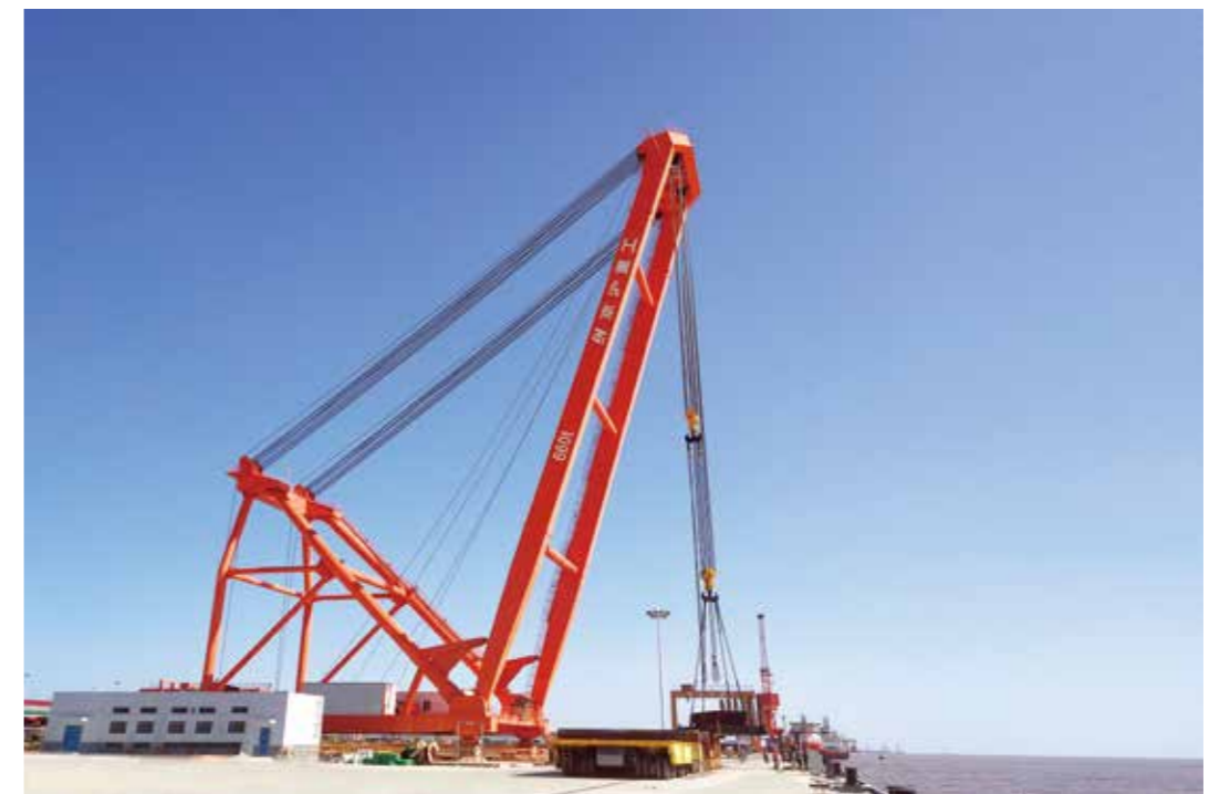
京沪重工660t固定式门座起重机 Beijing-Shanghai Heavy Industry 660tons Fixed Portal Crane
