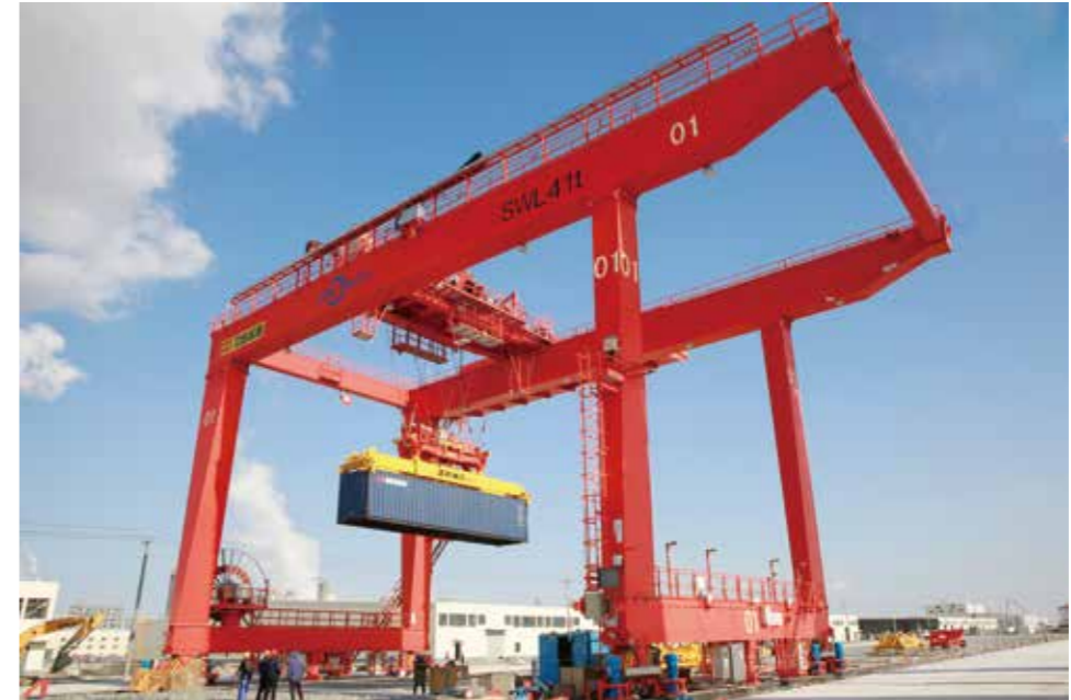
浙江石化自动化轨道式集装箱门式起重机 Automatic Rail Mounted Container Gantry Crane for Zhejiang Petrochemical Industry
