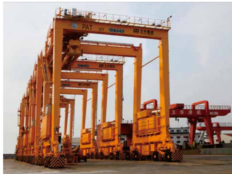
出口泰国轮胎式集装箱门式起重机 Rubber Tire Container Gantry Crane Exported to Thailand
